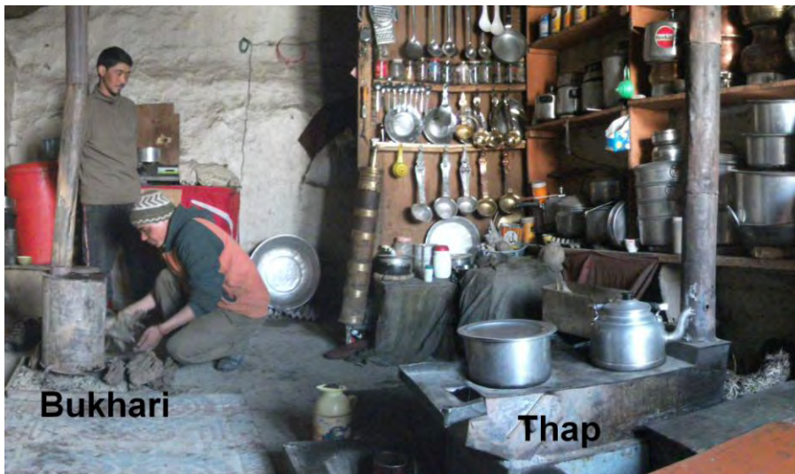
A Non-PSH family near Bodh Karbu. Bukhari (left) is used primarily for heating; Thap (Right) is used for cooking- While both can heat and cook to some extent the design is optimized for one purpose. Non-PSH families are often forced to use both during winters.
